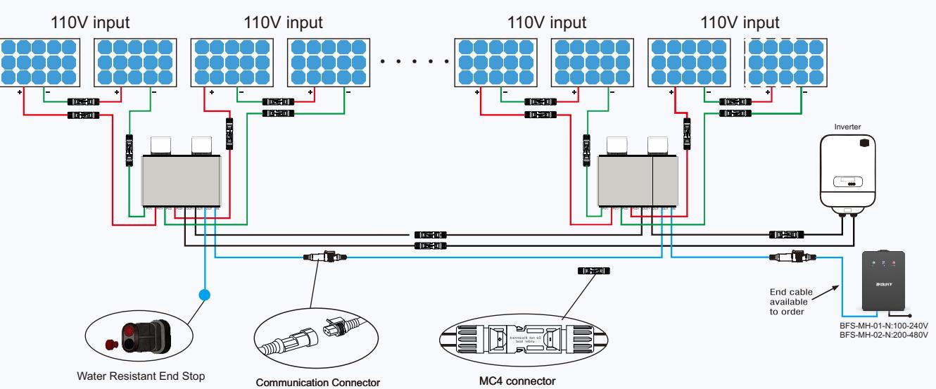
Each BFS-A1/BFS-A2 device can accommodate solar modules with a total max output of 1500V. The modules connect in series as the solar string links to the inverter as will be stated in the PV design. The BFS-A1/BFS-A2 and Rapid Shutdown Monitoring Device are connected via communication cable.
